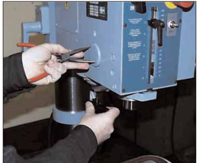
Picture 4. Removing the spring case
